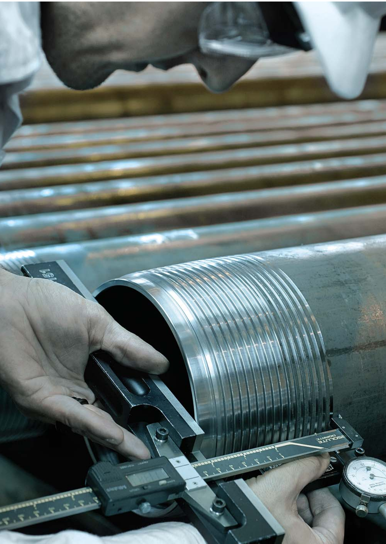
Commercialization of new premium connection technologies entails previous fulfillment of advanced performance evaluation tests. A qualification procedure usually takes around 800 hours to complete.
