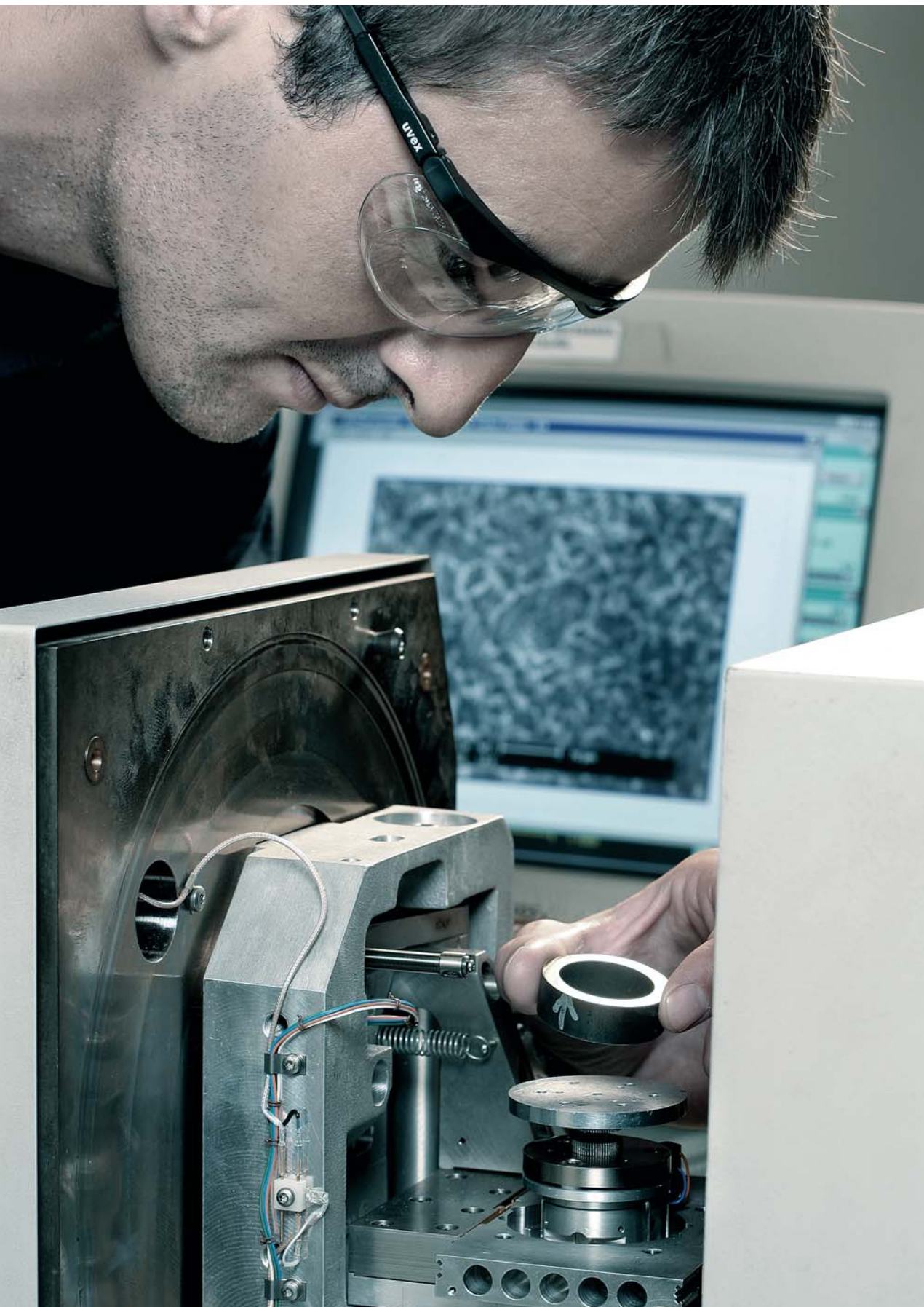
The Scanning Electronic Microscope (SEM) allows us to identify on samples if there is any defect on the steel manufacturing or during the pipe manufacturing process through magnifications showing the contained elements and their amount.
