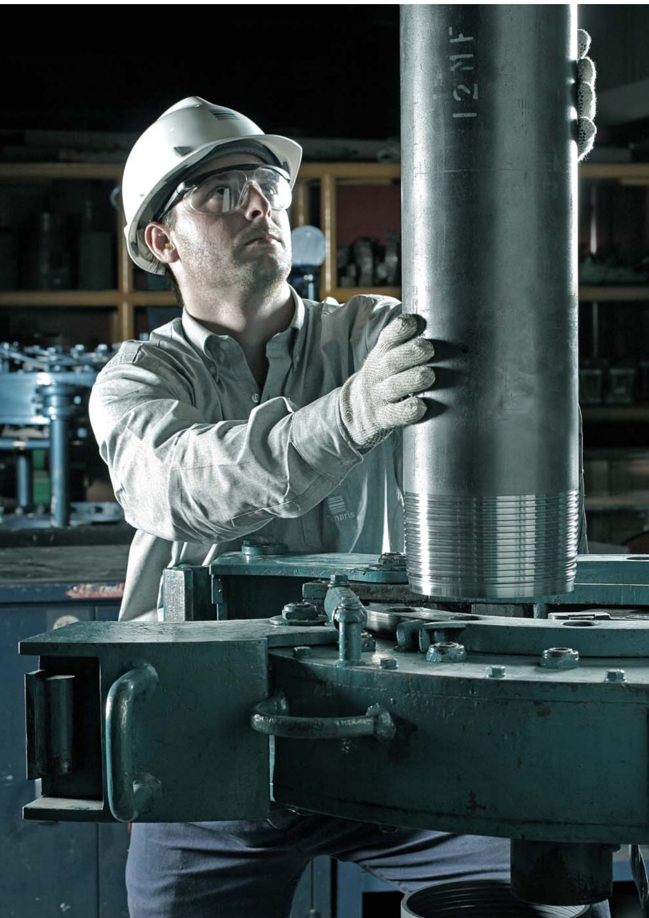
Tenaris reproduces field conditions at its full scale testing facilities as closely as possible. OCTG and connections are rigorously tested to confirm their resistance to collapse, burst, fatigue, torque, compression and combined loads. Bending and post-welding properties are also measured for ultra-deepwater line pipe.
